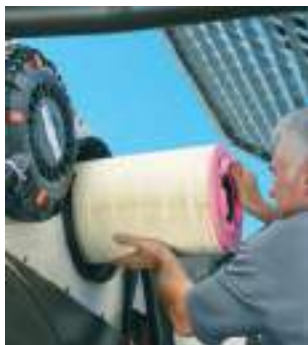
Air filter change without tools
