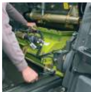
Quick removal and installation of the corncracker
