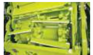
V-MAX chopping drum with knives removed.
